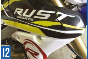
revealed in-mould fixings that would need to be cutaway to fit the Acerbis light. The right thing to do here is to buy a YZ-type guard instead (£19.99 from Acerbis) and fix the light to that. You'll also need to sort connectors for the wiring – again, something I didn't have to hand. In the end, the ghastly steel OEM framework had to go back on to ensure full legality for the W2D.
