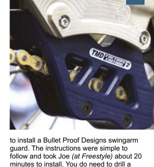
to install a Bullet Proof Designs swingarm guard. The instructions were simple to follow and took Joe (at Freestyle) about 20 minutes to install. You do need to drill a hole in the swingarm and tap a thread and that may not be possible for everyone if they are lacking in the tool department but the end result is worth the effort.
