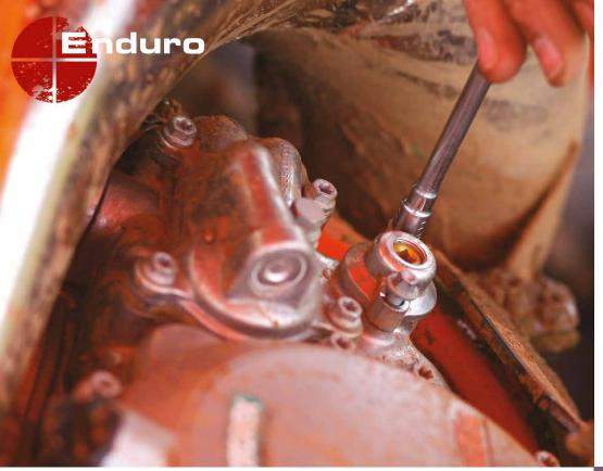
valve) or a red spring for more aggressive performance. Changing the spring takes about three minutes. Just lay the bike on its side, remove the two bolts that hold the cover over the springs, remove the spring set and swap to the spring of choice, then re-assemble. Easy!
